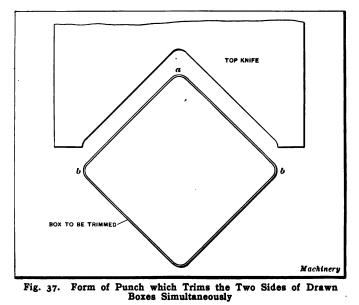
such as brass or aluminum but is liable to cause trouble when trimming steel, because the corners are so hardened, as the result of drawing, that the top corner a might split from the strain of the cut, unless the box were annealed for trimming. The fixture for indexing and supporting the work is similar to the form illustrated in Fig. 36.
